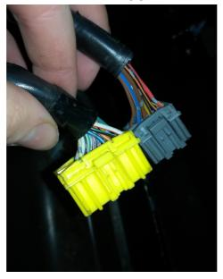
1. You'll notice the mounting bracket is different and the terminal plugs are mounted reverse on the Cappuccino ECU compared the AZ-1, this is not a problem.
