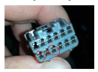
Close the terminal locks, plug the terminals in your Cappuccino ECU and put it back in place. I took out the white plastic wire guide for an easier install, and basically just left the ECU unbolted since it'll be held in place by the mounting plate.
